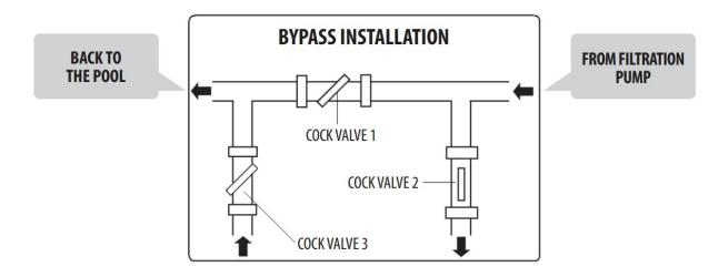
Close the cock valve 1 completely and open the cock VALVES 2 AND 3 on the inlet and outlet lines of the heat pump, respectively. At these conditions there is the maximum flow through the heat pump. Put the heat pump into operation in the heating mode. Wait until the value of pressure read on the pressure gauge stabilizes. The correct pressure setting should be within the range of 21 - 35 kg/cm<sup>2</sup> (bar).
