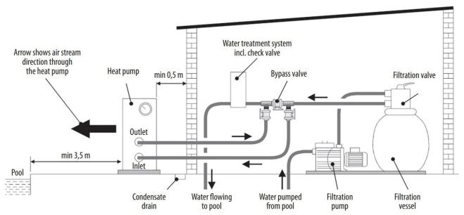
**NOTE:** The manufacturer supplies the heat pump only. Other components shown on the figure comprise the parts of appropriate water supply circuit and shall be provided by the heat pump user or installer's firm.
