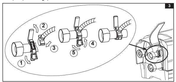
3. Unscrew the air valve cap on the spa tub to reveal the stem in the up position for inflation. Insert the other end of the inflation hose (7) into the valve and turn to the right to lock it in position (see drawing 4).
