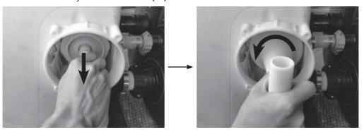
**5.** Pull out the electrolytic cell and place it in a container, pour kitchen grade vinegar into the container to soak the titanium plate for about one hour until no deposits remain.
